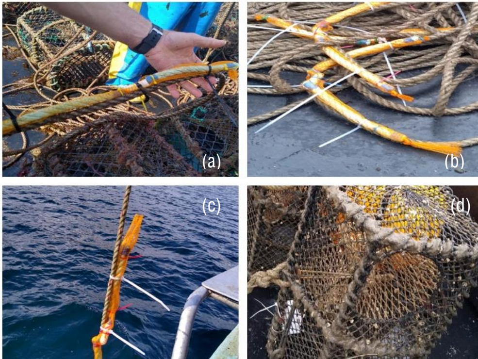
Figure 5.2. (a-c) Attachment of DST tilt sensors to groundline. The sensors are the small white cylinders in between two sections of rope within the orange netting. The whole attachment was neutrally buoyant; (d) the sensor is in the white housing attached to the inside of the creel
