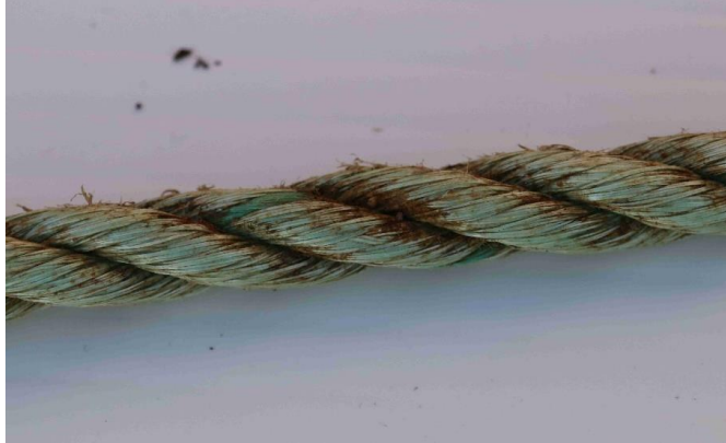
Figure 4.4. Seasteel rope used in trial showing typical levels of minor abrasion after over one year of use. Breaking load 93% of new equivalent
