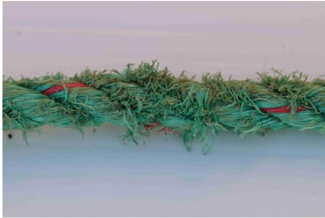
Figure 4.5. Polysteel rope used for the trial showing heavy abrasion after over one year of use. Breaking load 88% of new equivalent
