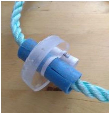
Figure 5.4. Set up of sensor to measure line movement on the seabed. The clear disc is 60mm diameter and can rotate around the line
