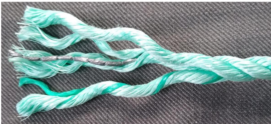
Figure 3.1. A sample of Seasteel sinking rope with the strands separated to show the thread of beaded lead
